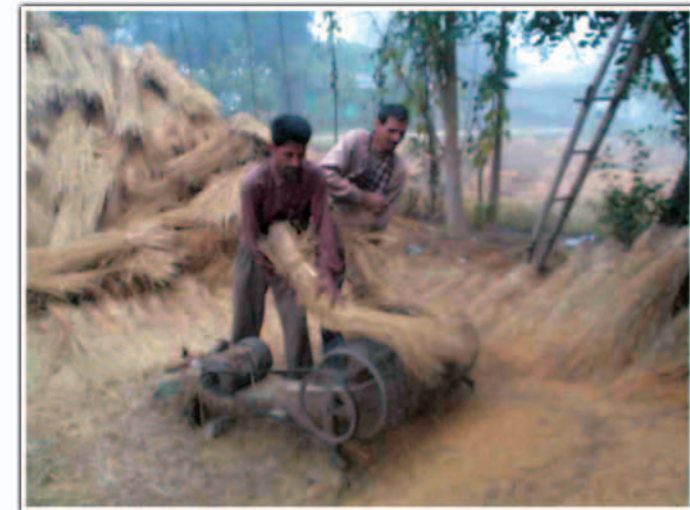
Farmer of Chitwan district Mr. Roman Neupane has come up with Electric Thresher-cum puddling/planking Machine
